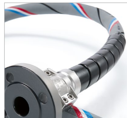
KSS Anti-Kinking Spiral with suitable Spannloc KSS clamps. Patented system for tightly bent hoses – protects the stressed area directly behind the coupling (see ELAFLEX Information 2.09 E)
