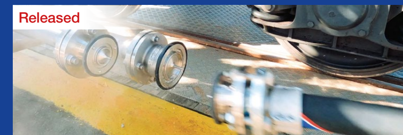
After an emergency disconnection the coupling separates and both valves close immediately.
