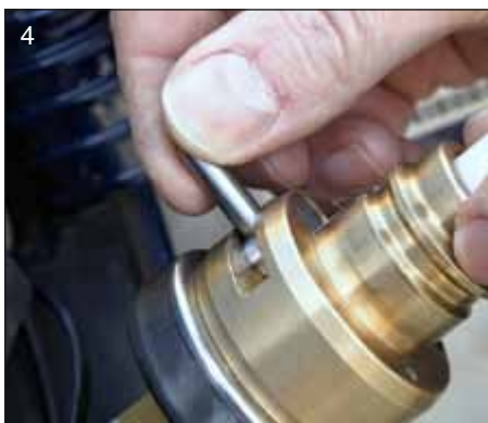
Move lever of adapter in upright position to connect both parts.
