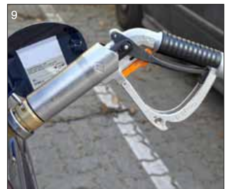
To disengage, follow steps 1-8 in reverse order. Attention - when uncoupling, a small amount of gas is released.
