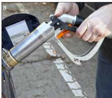
Latch nozzle lever, start refuelling. Safety feature: the lever of the adapter can not be moved during the refuelling process, the adapter can not be removed.
