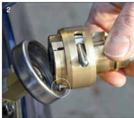
Hook the two bolts of the adapter into the collar of the DISH connector.
