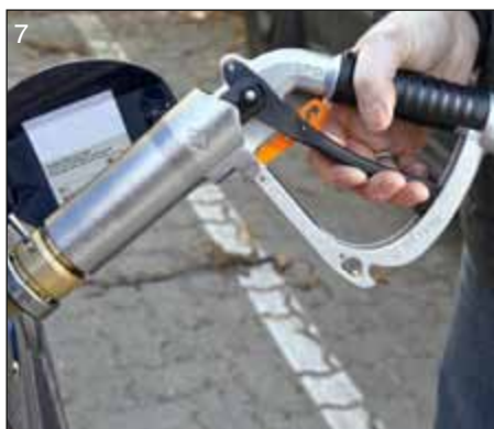
Pull nozzle lever to couple and engage the EURO nozzle.
