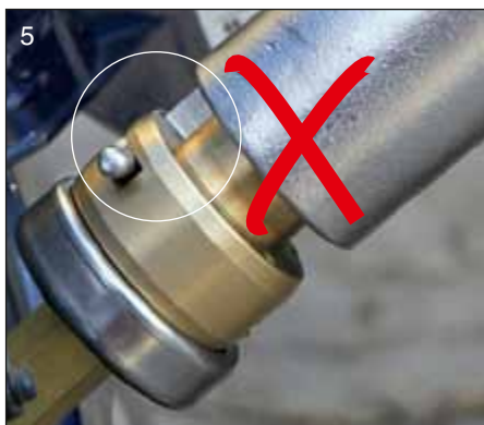
Safety feature: with lever in closed position the nozzle can not be coupled.
