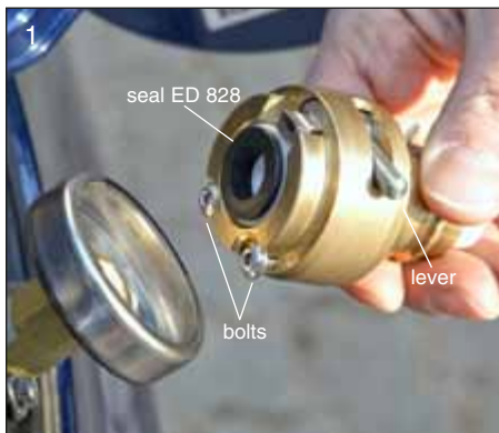
Right: Adapter EURO-DISH Left: vehicle sided DISH connector
