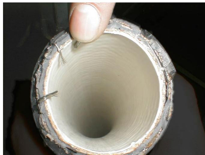
Shorten copper strands that they extend ca. 10 mm into the hose. Bend strands inside in longitudinal direction.
