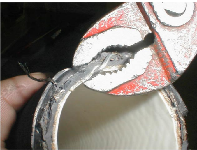
... to avoid damages to the hose tail during assembly.
