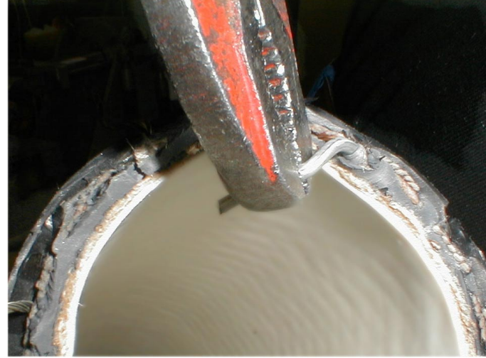
Bend helix inside with pipe wrench. Press the pointed end of the helix close against the tube ...
