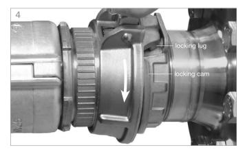
Lead female coupling with its locking lug to the locking cam of the male coupling. Do not use tools, hand force is sufficient.
