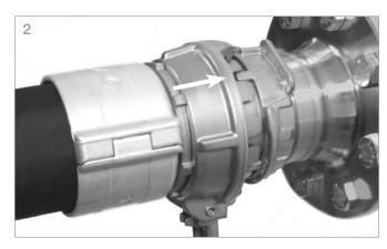
Join both coupling parts - recesses of the female coupling into bars of the male coupling.
