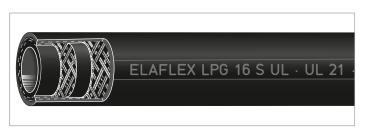
Working pressure max 350 psi (25 bar), burst pressure > 1750 psi (120 bar). Safety factor 5:1. Electrical continuity:  $\Omega$ -type to ISO 8031.
