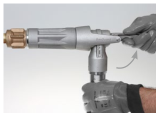
Actuate lever until held in cam open position. Start refueling.
