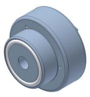
'H' Nose Piece (H) Common for attended sites. Flowrate up to 60 l/min at 12 bar system pressure. Release volume 1.7 cm<sup>3</sup>. Lower lever force than 'E'.
