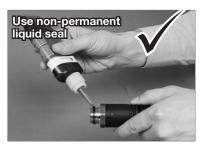
After connecting to the hose assembly, an operational test shall be performed. It is essential to examine that the nozzle, hose connector and swivel are tight under pressure and do not leak – e.g. by external application of foaming agents.
