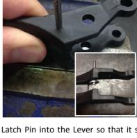
Hit the Latch Pin into the Lever so that it slightly protrudes out the other side of the first 'ear'. You can then put the washer over the pin.
