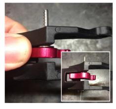
Align the hole in the latch with the Pin and hit through enough so that the pin is flush with lower side (in the picture) of the Latch.
