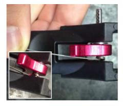
With the hook of the spring in the groove, align the coil of the spring with the hole in the Latch. Once it is aligned carefully hit the pin in completely. Test Latch to see if it moves freely forward then returns.
