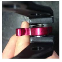
Fit the top 'hook' of the spring to sit in the groove. Make sure the 'tip' of the hook sits on the washer side of the Latch.
