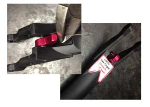
Cut the long section of the spring so that it sits in the recess. Clean the back of the Lever and attach the sticker.
