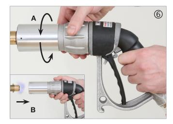
Once gas is discharged, turn connector nut anticlockwise (A). Nozzle can now be removed (B). A small amound of residue gas is normal.
