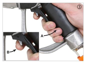
Pull lever back (A) and latch as shown (B). The system is now secure and you can remove your hands from the nozzle.
