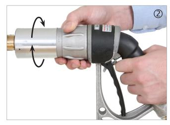
Hold the nozzle with one hand while rotating the connector nut 20° - 55° in a clockwise direction with the second hand.
