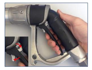
To unlatch Lever, squeeze Lever and latch will automatically unhook itself from latch pin.
