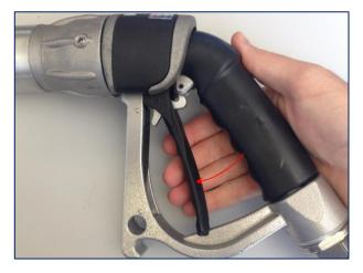
User can now safely lower the lever to close the valve. Caution: A small discharge of gas is released from connector nut, please keep hands away. Once gas is dispersed the nozzle can now be removed.
