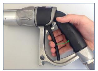
Once the nozzle is securely attached to the fill point, pull Lever open to allow flow.
