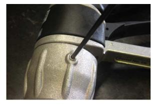
Carefully remove Grub Screw with 3mm Hex key
