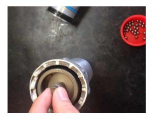
Insert the Nose Piece into the Connector Nut in the orientation shown.
