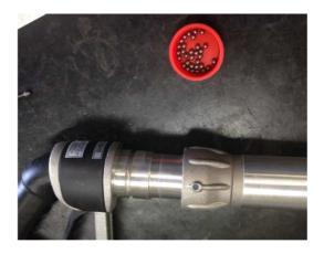
Once all the ball bearings are removed, the Connector Nut can be taken off.
