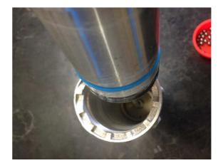
Apply a small amount of Nulon lubricant or similar to the Slide Sleeve. Guide the Nozzle and Slide Sleeve into the Connector Nut.
