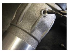
There will be residual Loctite which should be removed with a 5mm drill bit.
