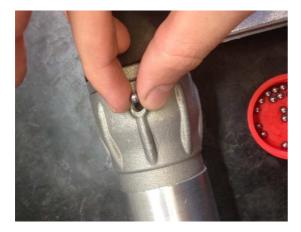
Re-insert the thirty-one (31) ball bearings into the hole on the Connector Nut.
