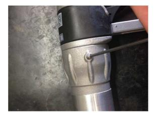
Once all balls are inside, apply a dab of locktite 262 or similar to the grub screw and screw until flush. Rotate Connector Nut to check for smooth movement.
